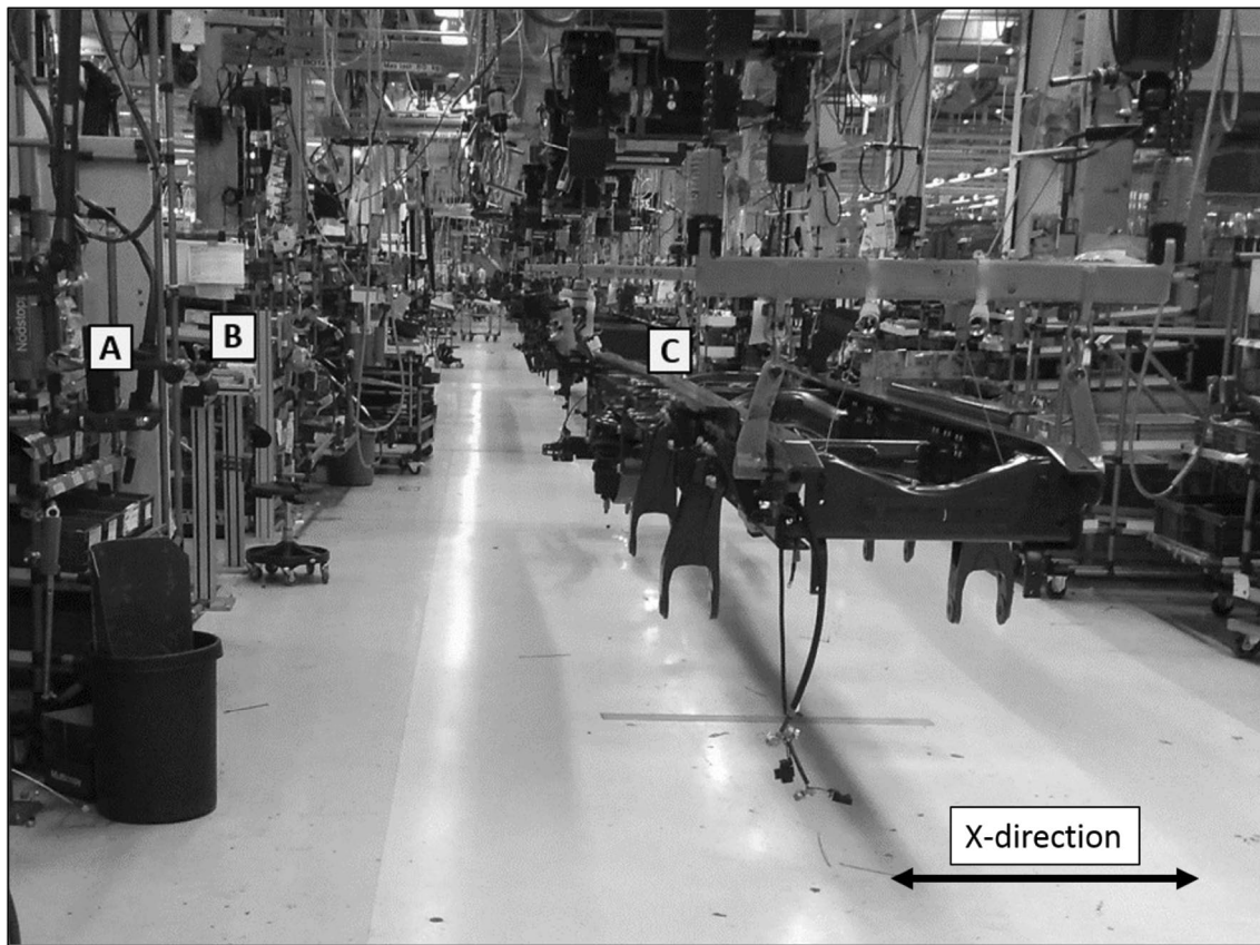
Fig. 2 Existing workstation. The gearbox insulator is moved from the rack (a) to a pre-assembly fixture (b) and finally installed inside the C-shaped frame (c)
