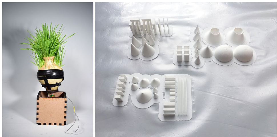
Fig. 5 Centrifugal force experiment set-up (left); 3D-printed moulds for making growing vessels for barrier experiments (right)
