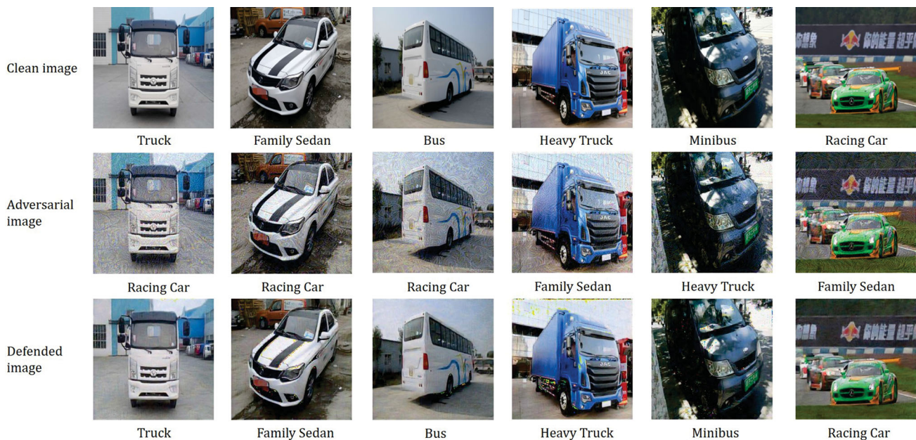
Fig. 5 Selected examples produced by DDAP. Labels below each image indicate the output classification.
