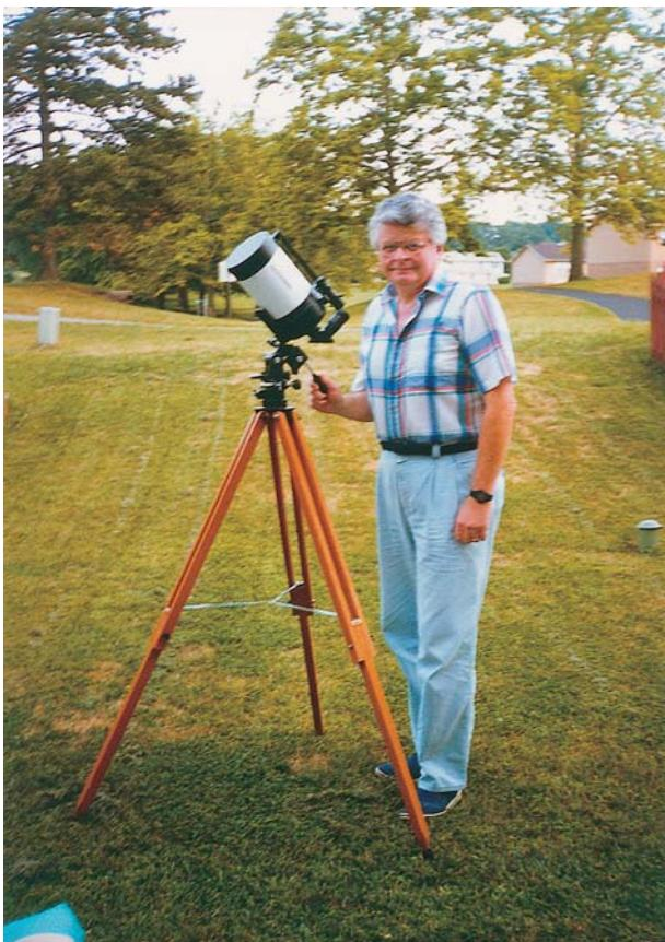
The author shown with his 5-inch Celestron Schmidt-Cassegrain optical-tube assembly mounted on an exquisite old Unitron altazimuth mounting with slow-motion controls. With excellent optics and a total weight of just 12 pounds, this highly portable instrument can go anywhere and is a joy to use. Photo by Sharon Mullaney.
