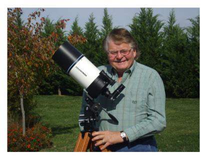
The author shown with his 5-inch Celestron Schmidt-Cassegrain optical tube assembly mounted on an exquisite old Unitron altazimuth mounting with slow motion controls. With excellent optics and a total weight of just 12 pounds, this highly portable instrument can go anywhere and is a joy to use. Image courtesy of Sharon Mullaney.
